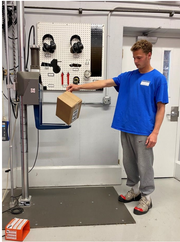
Image 1. Drop testing decoy packages to calibrate them before being sent on their data collection shipment.
