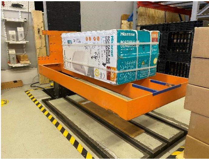
Image 3. ISTA Amazon 6B drop tests being conducted on portable AC units.
