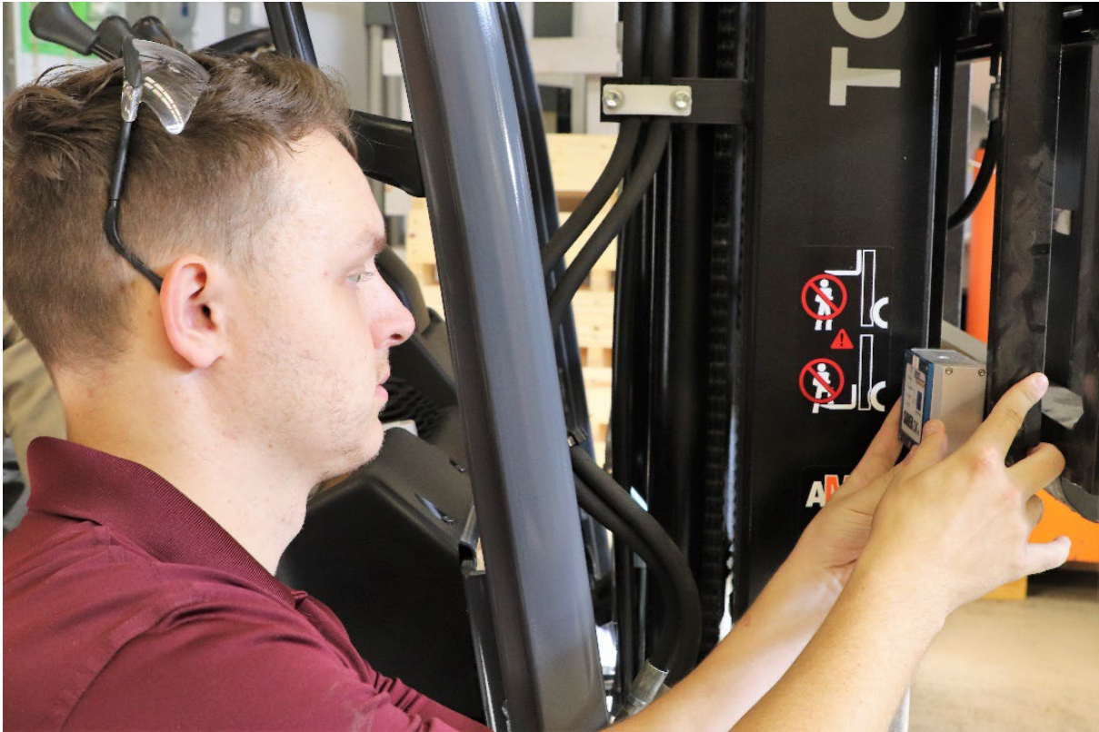
Image 2. Clark Sabbattus equipping a forklift with a sensor to measure the shock events experienced in various warehouse facilities
