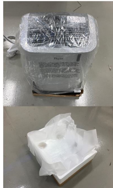
Image 4. Examples of bags and sheets used to protect the AC unit within the corrugated packaging.
