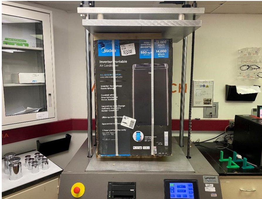
Image 1. Portable AC unit being compression tested during this undergraduate research project.
