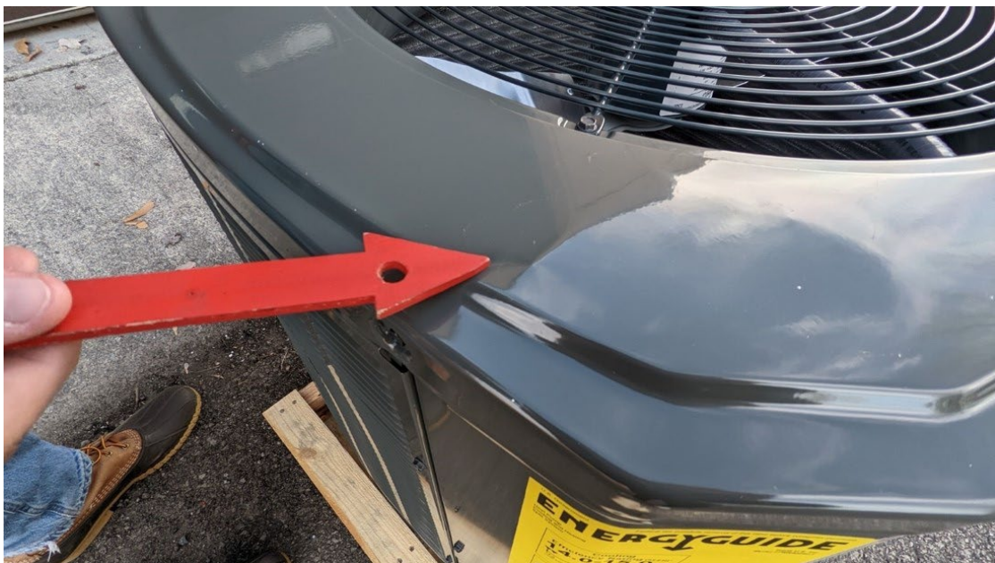
Image 3. Example of a dent to a Trane product which was incurred during testing.
