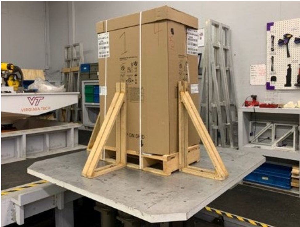
Image 1. Heat pump unit being vibration tested during this undergrad research project.
