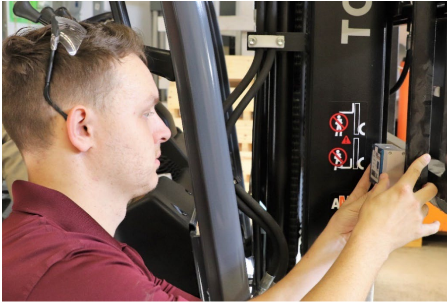
Image 1. Clark Sabattus equips a forklift with a sensor to measure the shock events experienced in warehouse facilities.
