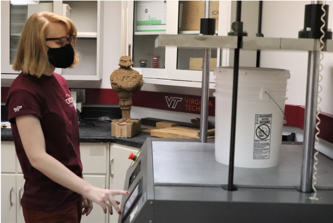
Image 1. Rosa Williams conducting compression testing of a plastic pail on the Lansmont Squeezer.
