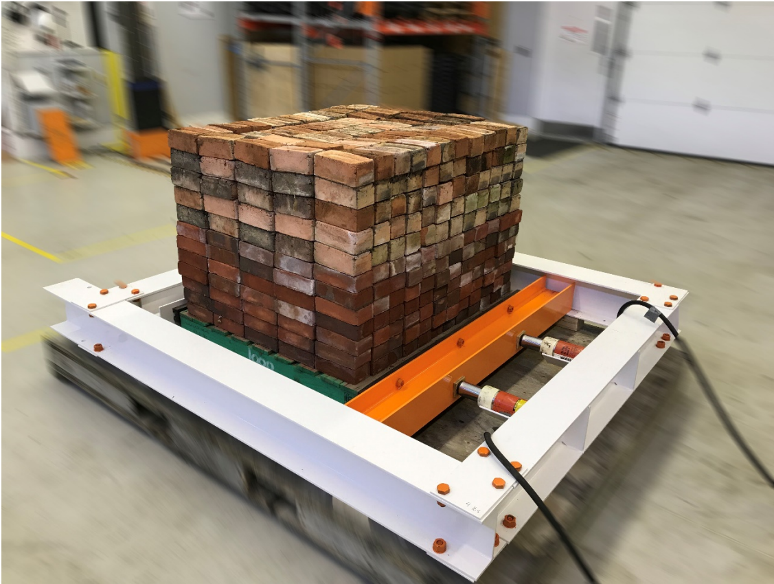
Image 3. Custom jig setup to mimic grab handling of a palletized unit load of bricks perpendicular to the stringers.
