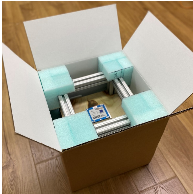
Image 2. Instrumented box used during the study.
