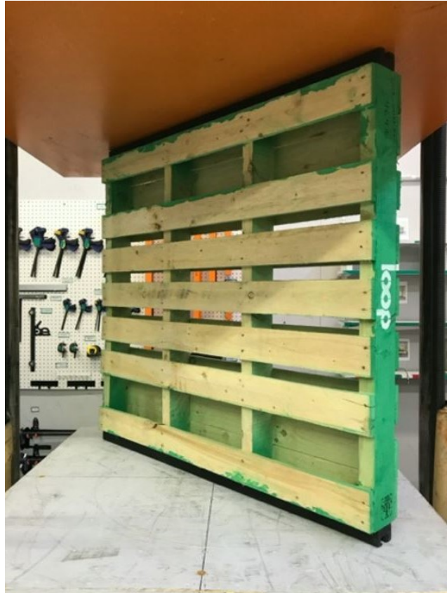
Image 2. Horizontal compression test setup in Tinius Olson machine — testing perpendicular to the stringers.
