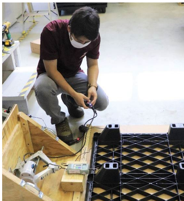
Image 3. Yu Yang conducting a Coefficient of Friction test on the plastic pallet.
