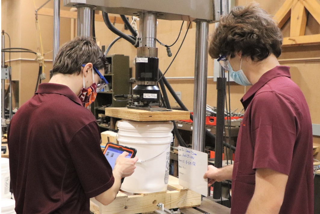
Image 1: Jordan Wells & Cameron Fischi conducting pail compression strength tests.
