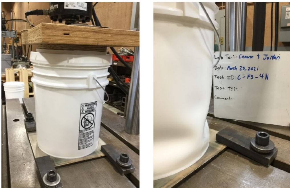
Image 4: Test setup picture showing the (left) pail-to-pail connection and (right) example of pail failure.
