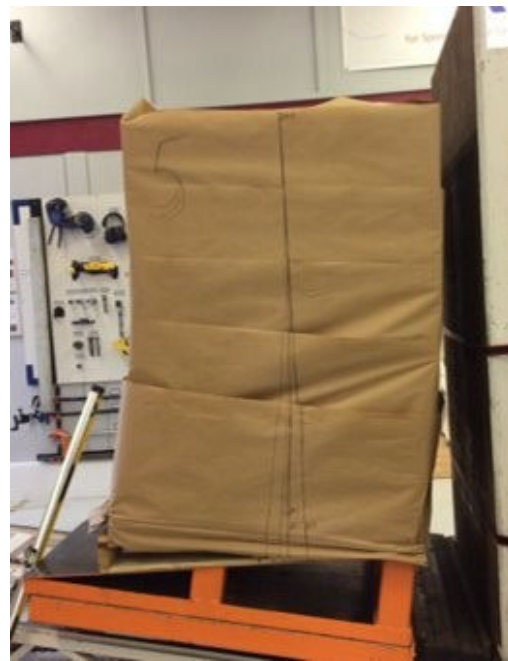
Image 2. Showing plastic-wrapped unit load failure (left) versus paper-wrapped unit load's performance (right) during incline impact tests.
