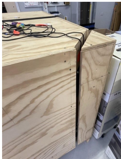
Image 3. View of corner containment testing area - the 2 load cells are located 10" from the top and bottom of the unit load.
