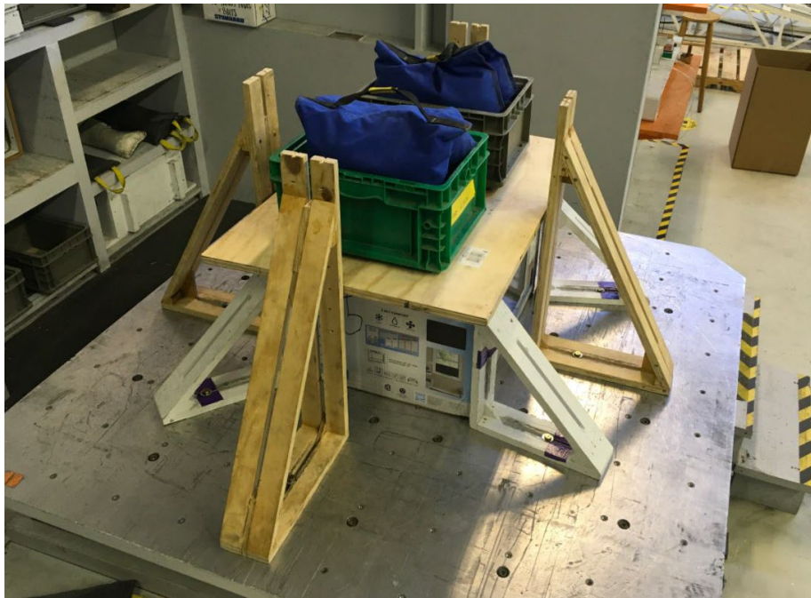
Image 1. Vibration testing of one of the AC units
