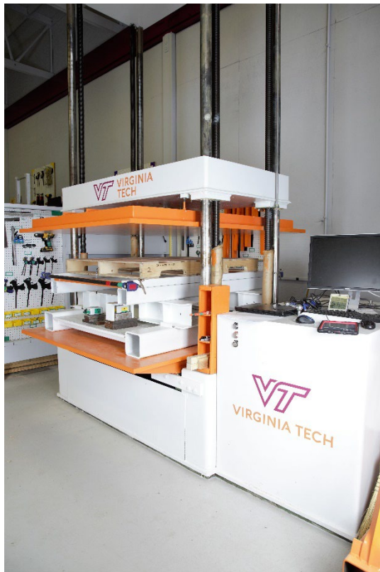
Image 1. a). Unit load tester in the distribution lab and b). upgraded software for the unit load tester
