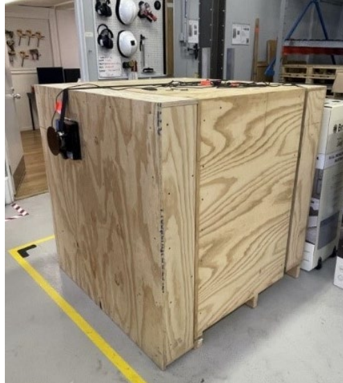
Image 2. Rigid test unit load with a length and width of 48 inches and a height of 50 ¼ inches constructed of plywood and lumber. Shows load cell located on side of unit load.
