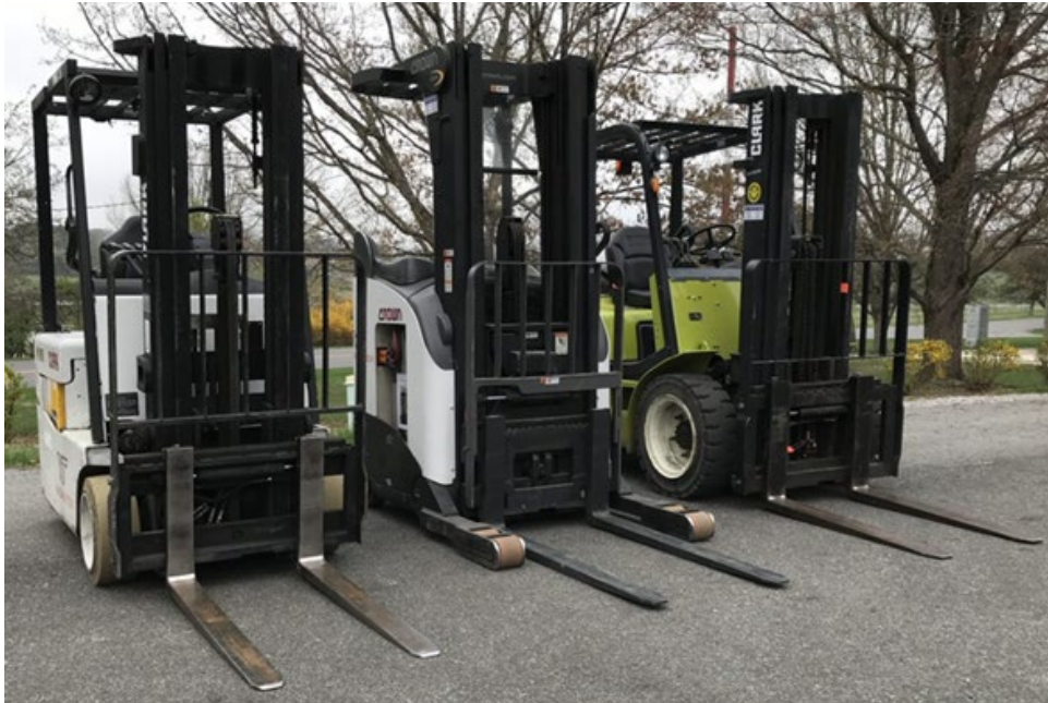
Image 1. Forklifts used in the study (left to right: gas, electric, reach).
