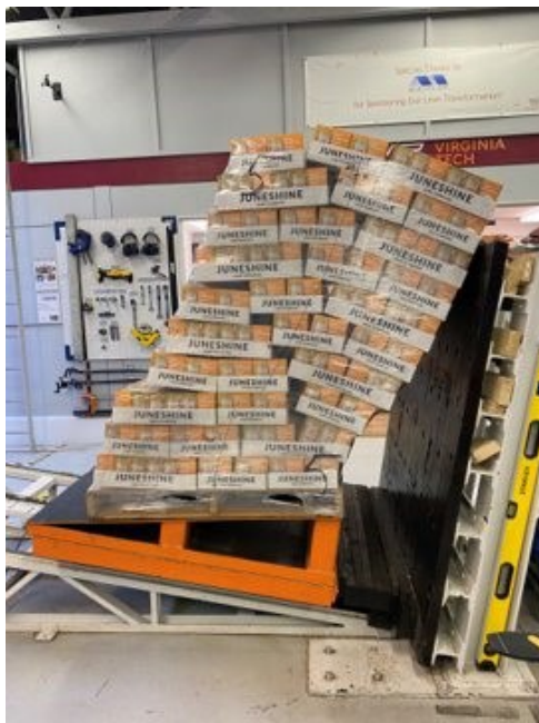
Image 2. Showing plastic-wrapped unit load failure (left) versus paper-wrapped unit load's performance (right) during incline impact tests.
