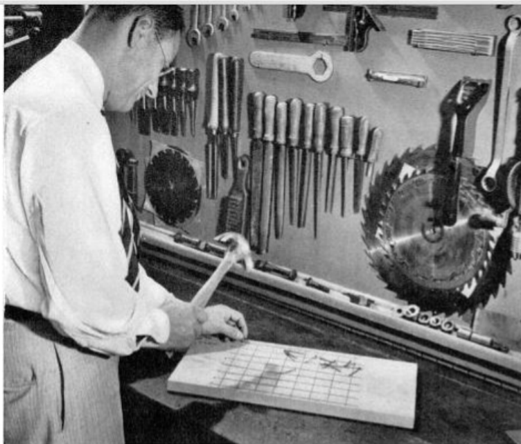
ONE TEST STARTS when Prof. Stern hammers different kinds of nails into a carefully graded board. Weeks to months later, he'll measure how hard they are to pull out.
