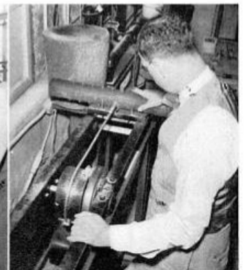
ONLY A CHARGING BULL, striking a wire fence, could match strength of yank that machine above gives driven fence staples. Cable on pendulum axis applies brutal tug.
