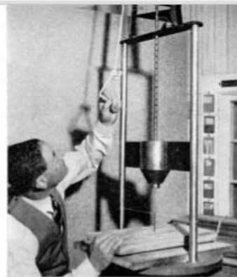
MEASURED BLOWS from the weight on this guillotine-like device reveal how readily a nail penetrates wood of known hardness. No human could hammer so consistently.
