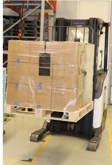
Photos: (left) Yu Yang Huang Qiu; (right) stretch-wrapped unit load of corrugated boxes being tested in the forklift handling condition.
