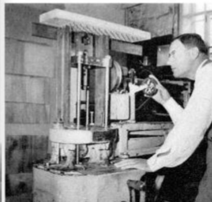
SLOW AND STEADY is the pull exerted on driven nails by the motor-operated claw of this machine. Motor runs at a constant speed and the machine measures nails' resistance.
