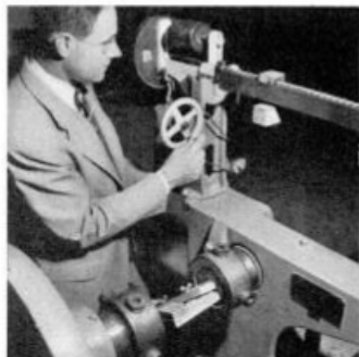
A TORTURING TWIST is applied to a furniture skid to find out exactly how much torque is needed to pry it open at its nailed joints. This test may save many a future table leg.
