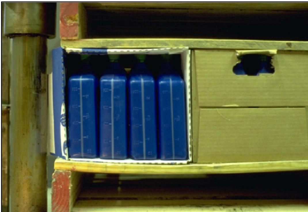
Figure 1.2 Non-uniformly distributed loads on packaging and pallet.
