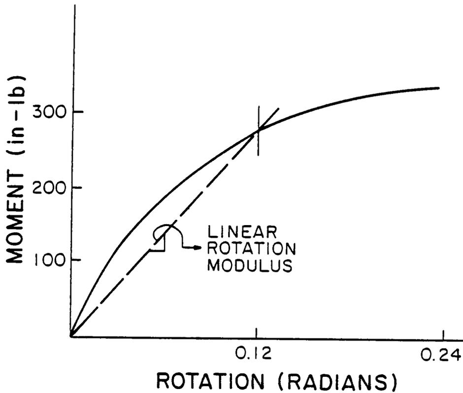
Figure 55. Typical moment-rotation curve. Estimated rotation modulus for rotation of 0.12 radians.
