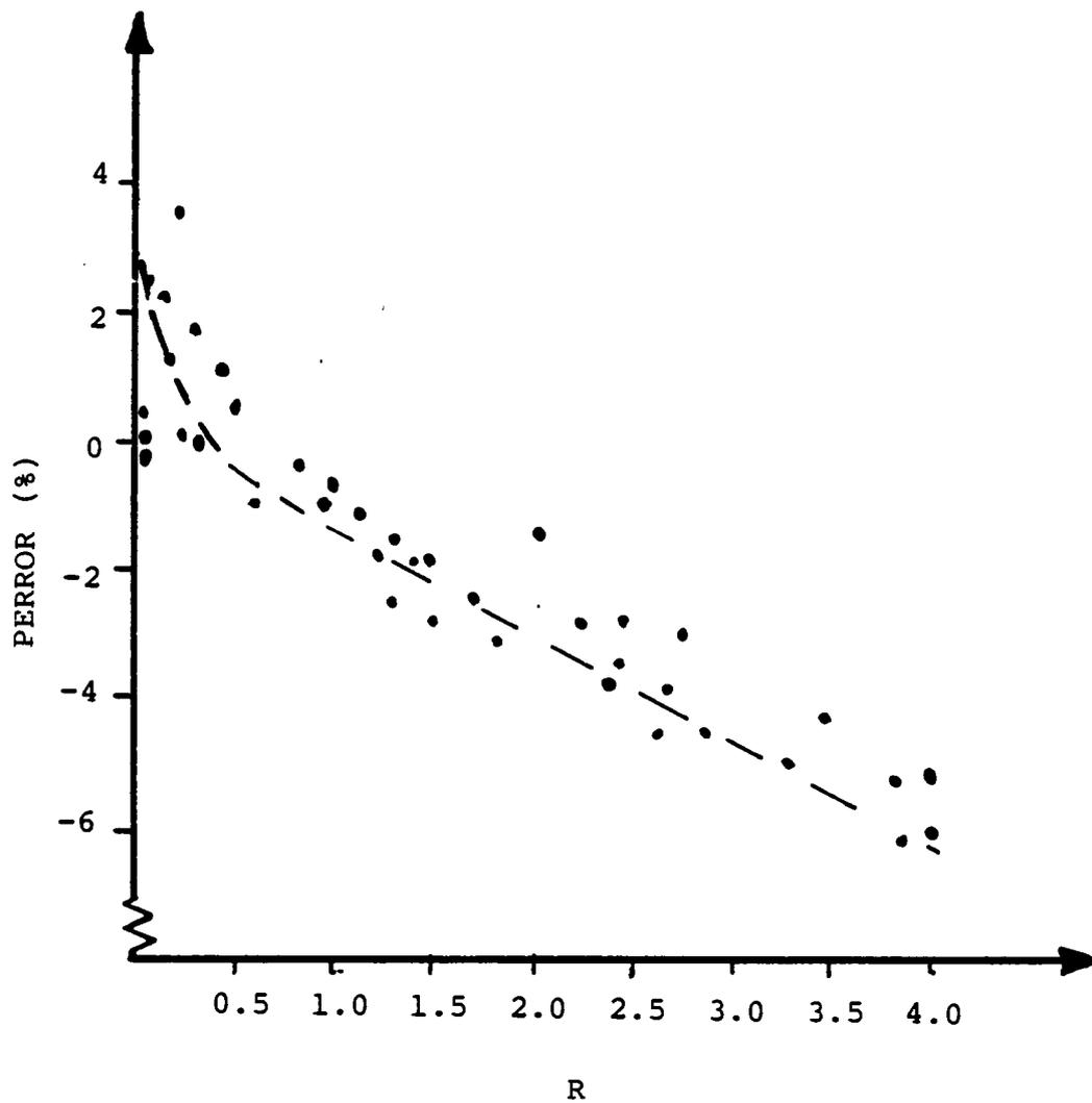
Figure 18. Four stringer pallet stiffness ratio vs ERROR with regression equation from Table 4.1 superimposed.
