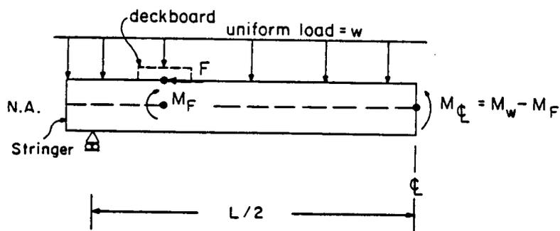
$F$  = load caused by deckboard-stringer shear,
