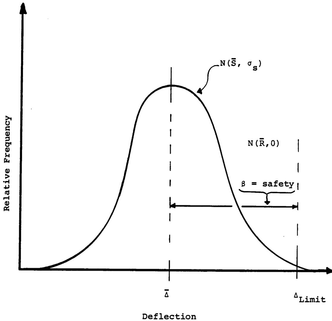
Figure 65. Illustration of serviceability limit state: analysis option.
