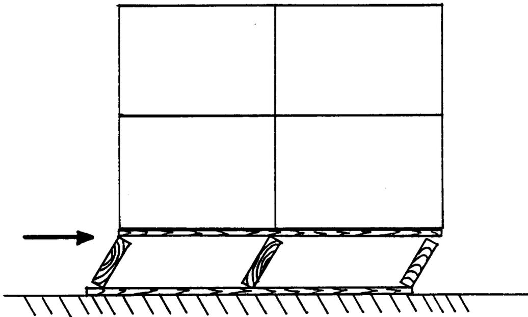
Figure 7 . Lateral collapse of a pallet.
