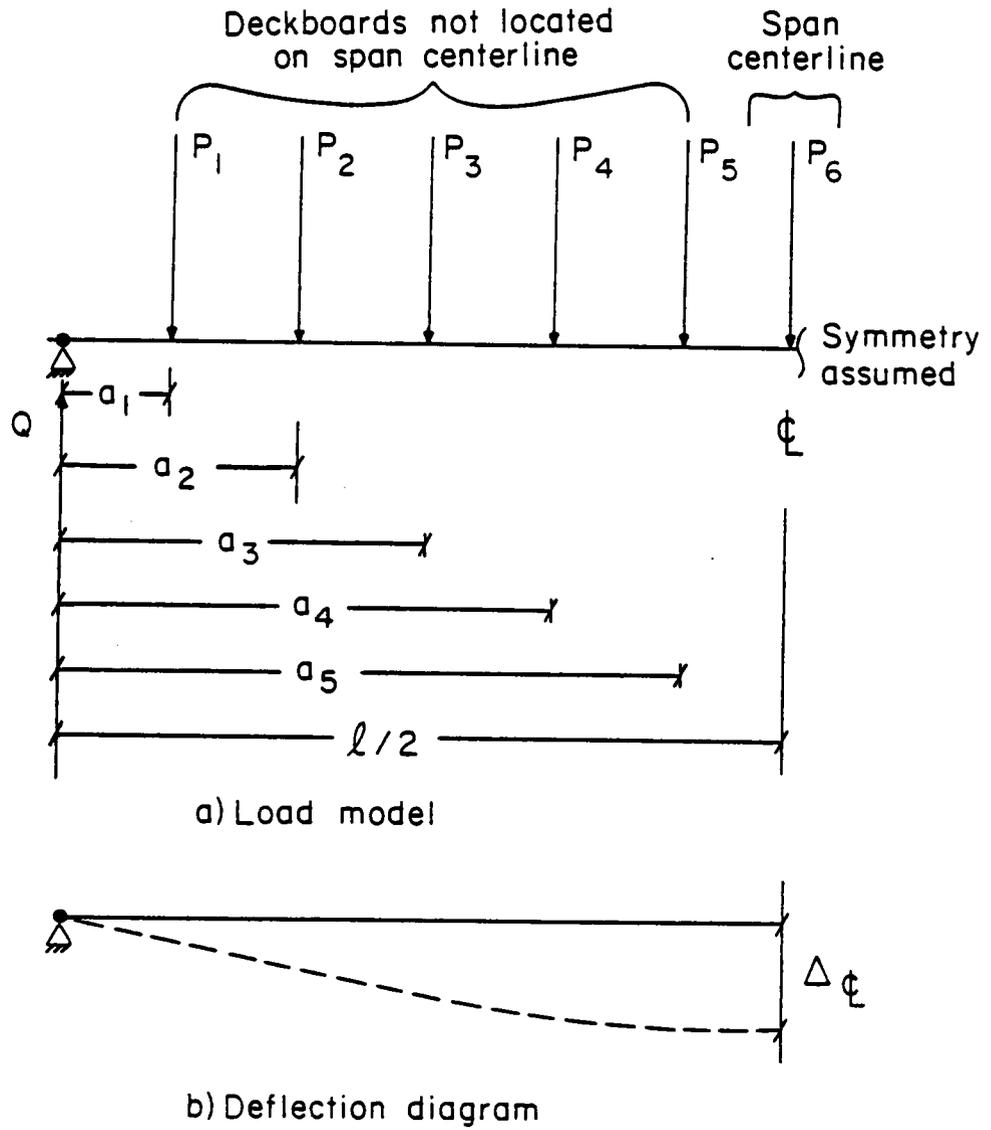
Figure 21. Diagram of symmetrically loaded stringer for computing stringer deflection RAS.
