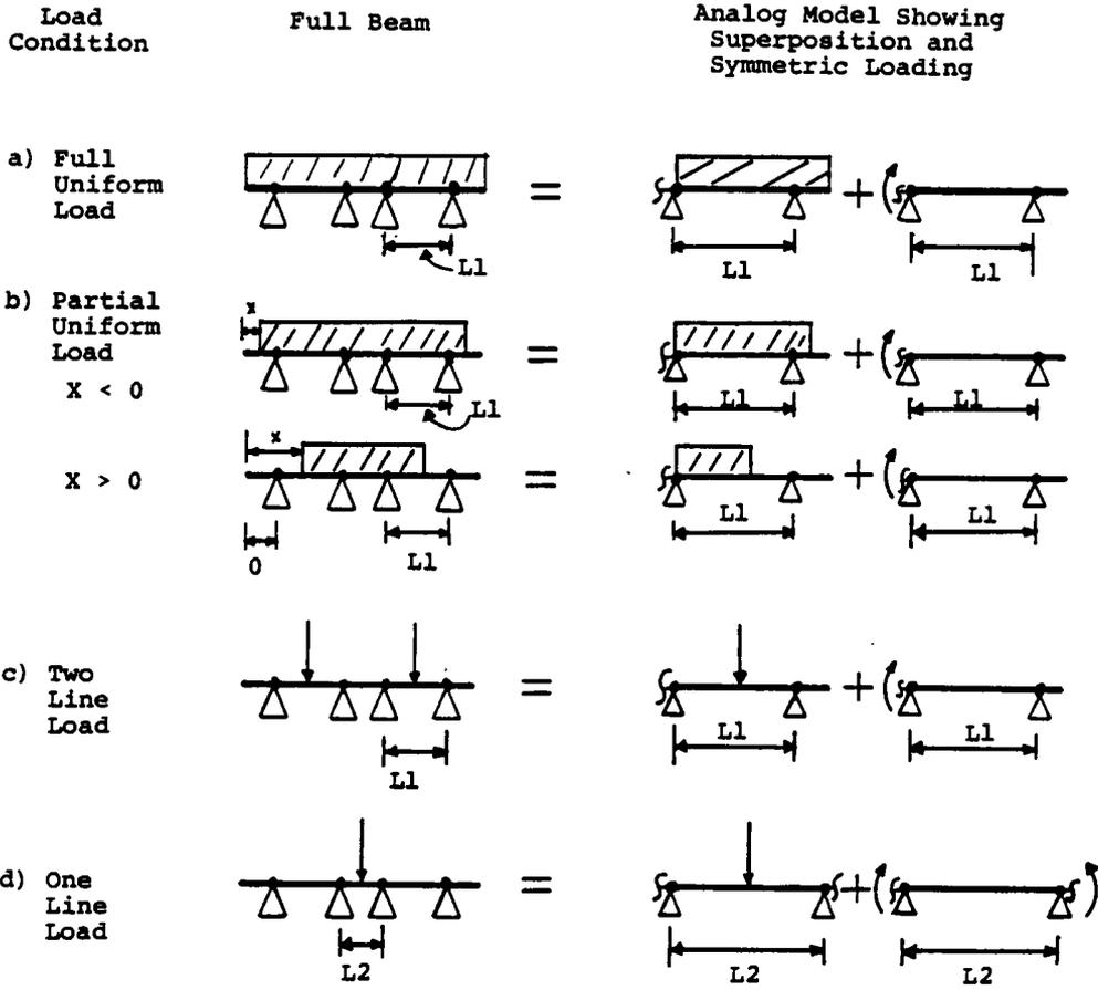
Figure 61. Stacked deflection analog models using symmetry and superposition.
