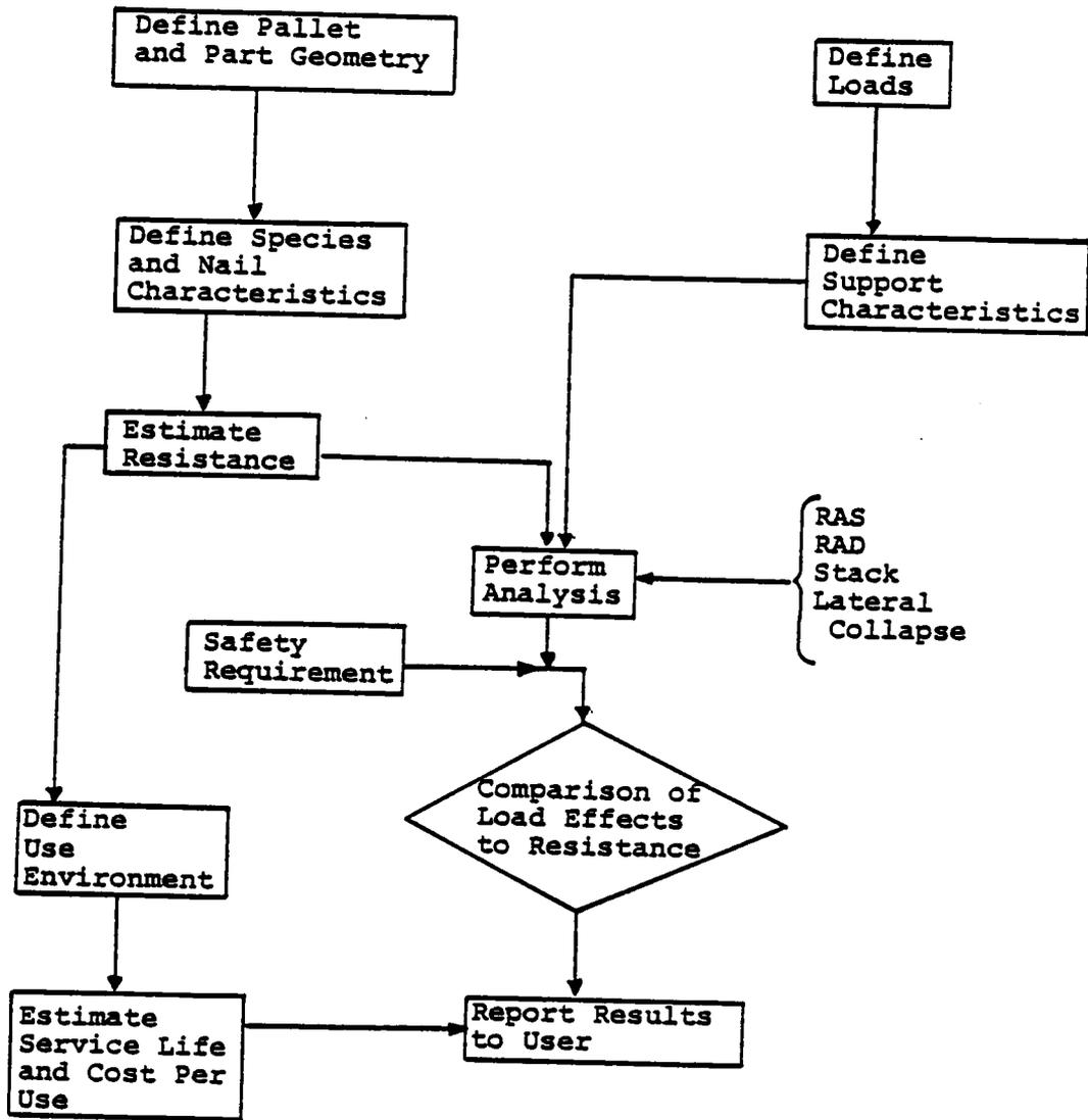
Figure 9. General flow chart of pallet design used in PDS.
