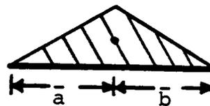
Figure 59 . Beam diagrams used to compute moments in stacked pallets.
