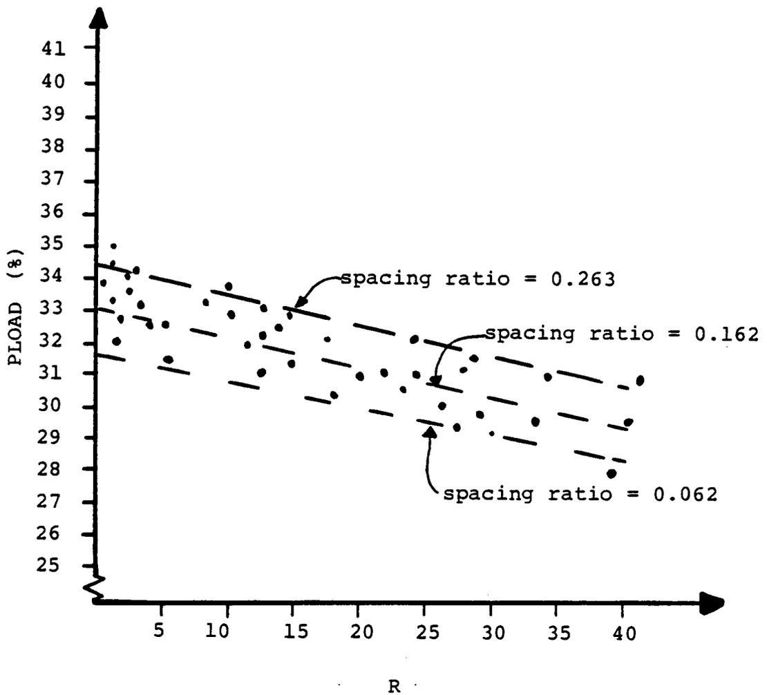
Figure 17. Four stringer pallet stiffness ratio vs PLOAD showing regression equation from Table 4.1 solved at three values of inner to outer spacing ratio.
