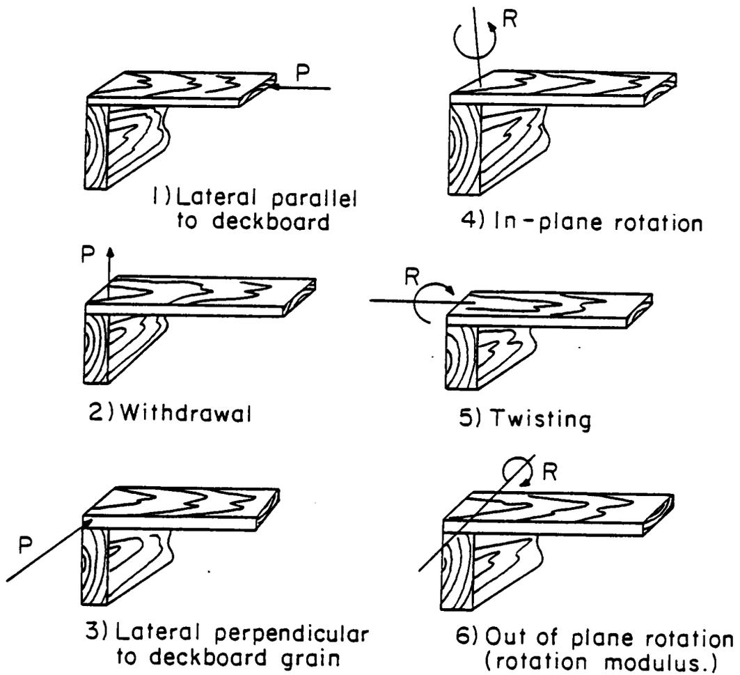
Figure 53. Six possible stiffness components of joints.
