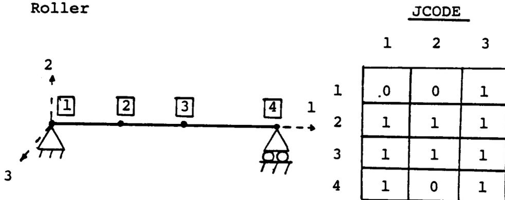
Figure 27. Example of use of JCODE to define constraints in a simple beam.
