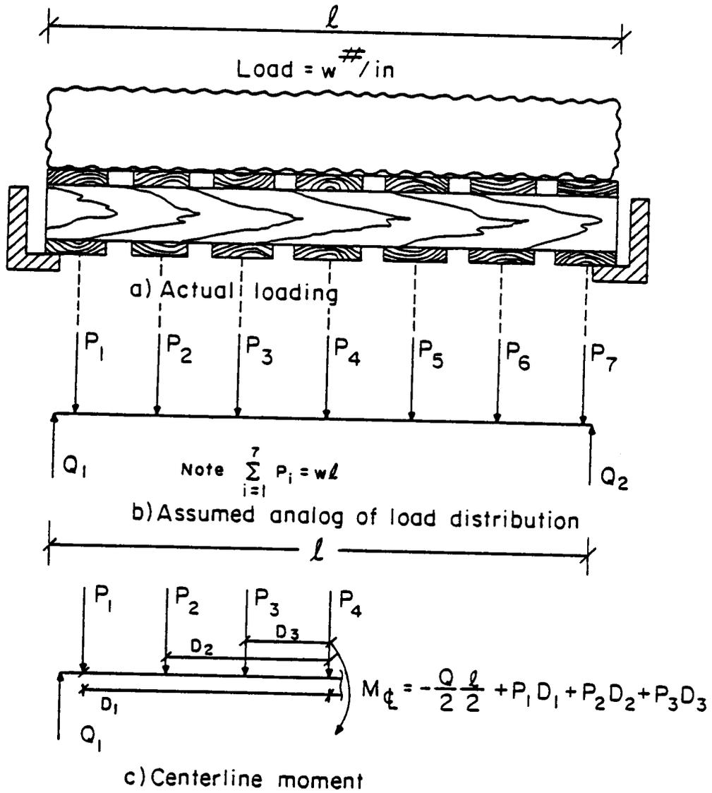
Figure 20. Load diagram for RAS uniform load.
