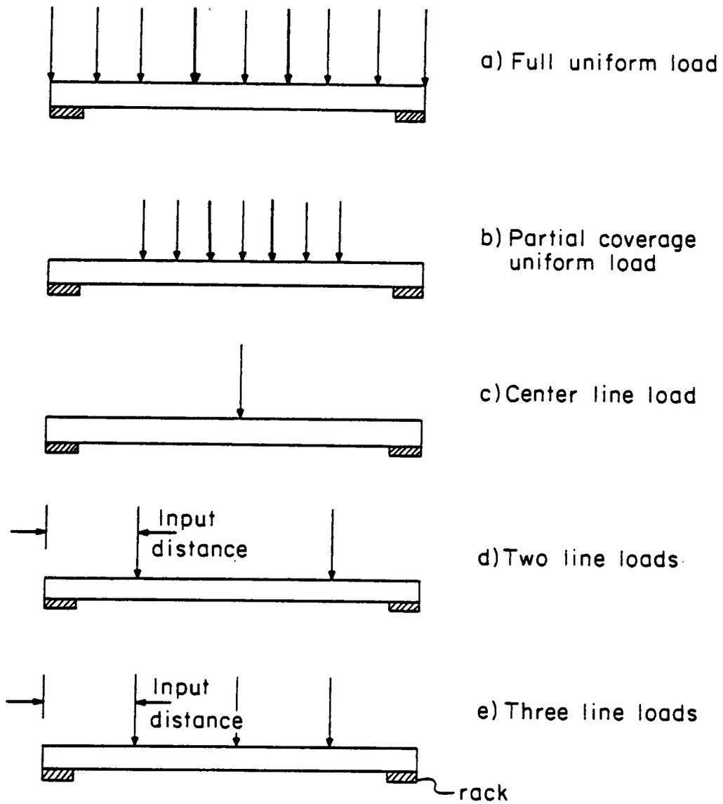
Figure 11. Analog load types analyzed by PDS.
