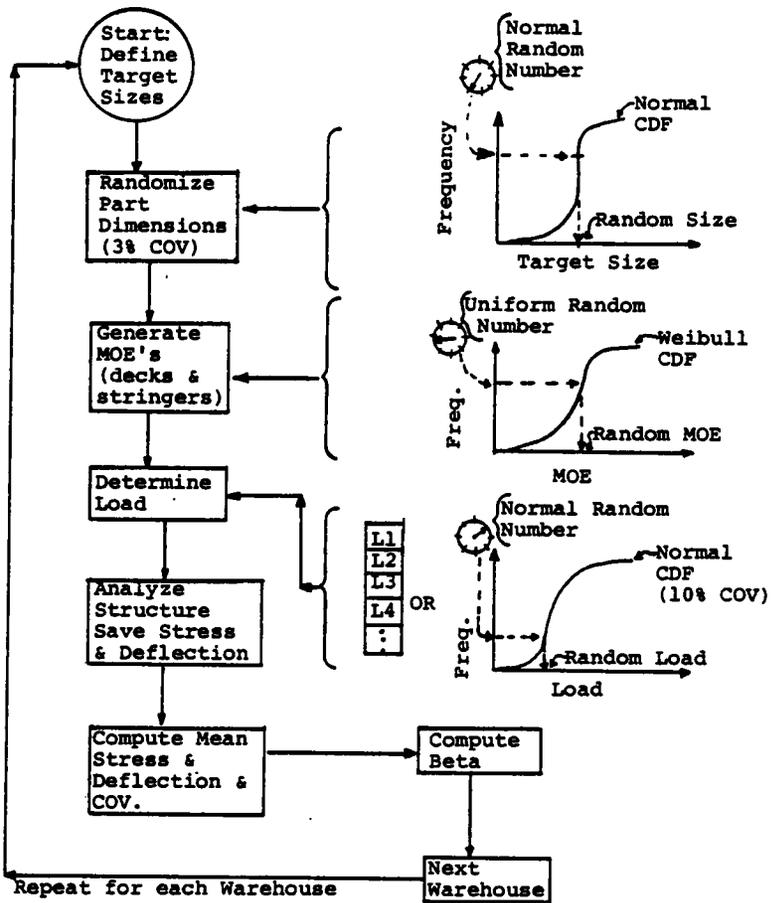
Figure 66. Flow chart of simulations to calibrate Beta.
