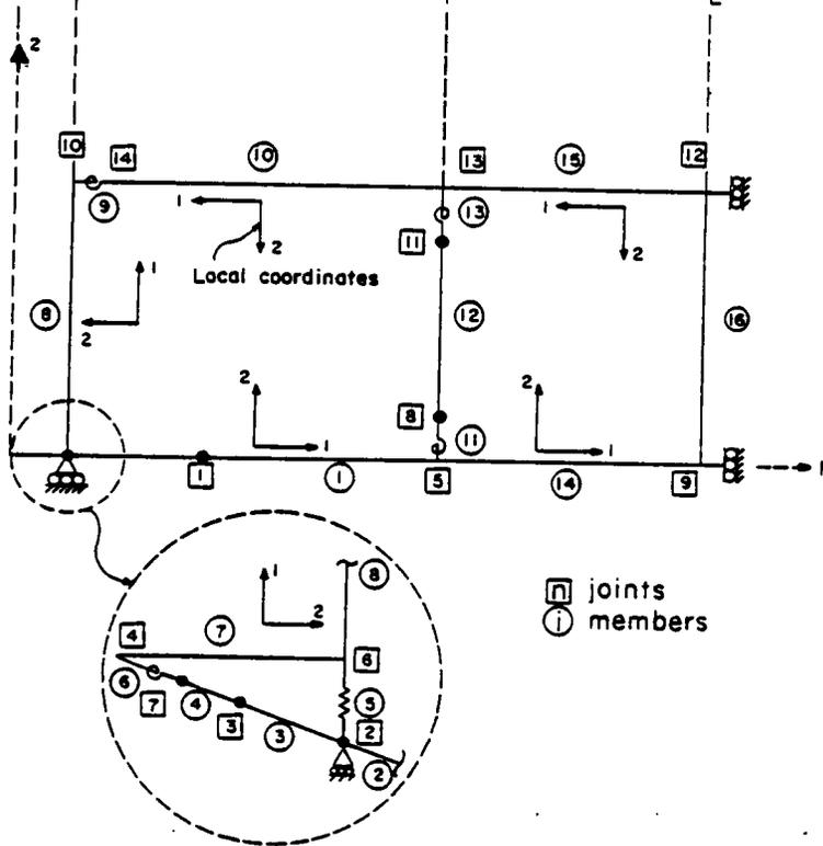
Figure 36. Analog model of RAD pallet
