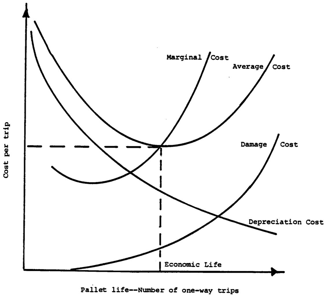
Figure 69. Pallet costs-per-use functions
