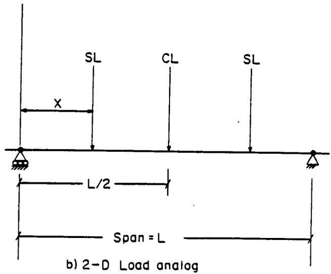
Figure 22. Analog model of RAS pallet loaded with line loads.
