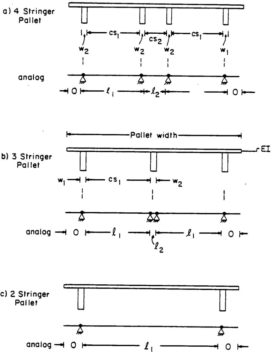
Figure 56. Analog models for rigid support condition.
