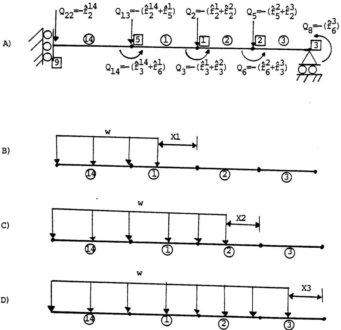
Figure 48. Load models for uniform and partial uniform loads for sling supported winged pallets. (a) equivalent fixed end forces ( $Q_i$ ), corresponding to degree of freedom for structure (see Table 5.1 for computation); (b) partial uniform load over member 1; (c) partial uniform load over member 2; (d) partial uniform load over member 3.
