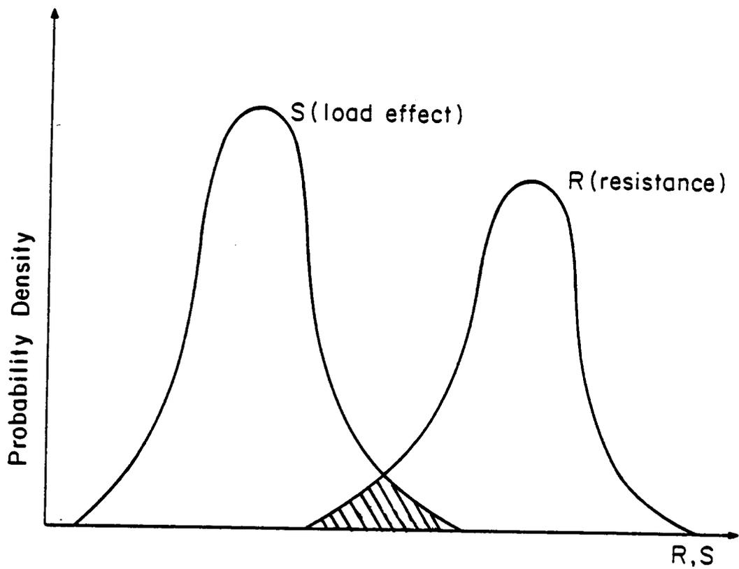
Figure 1 . Probability of failure.
