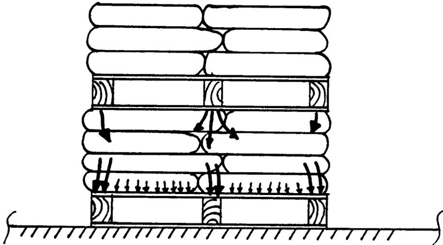
Figure 57 . Schematic diagram showing the assumed load transfer in stacked mode.
