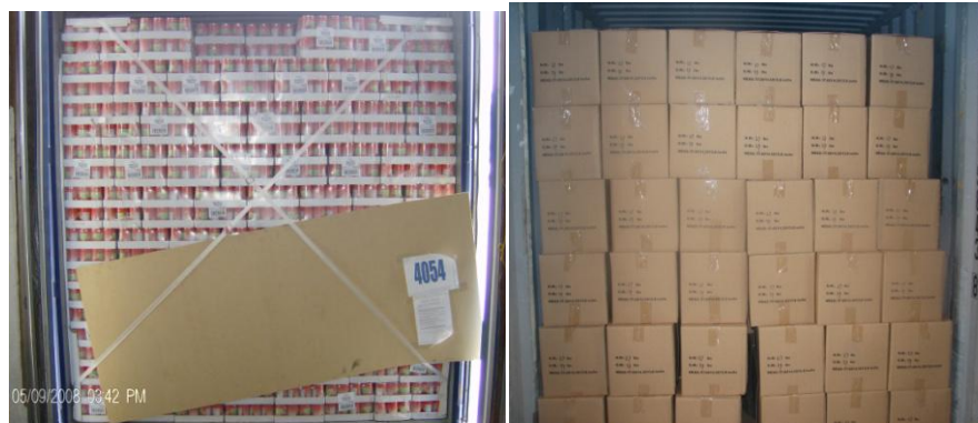
Figure 2-1 Boxes Floor Loaded in a Container
