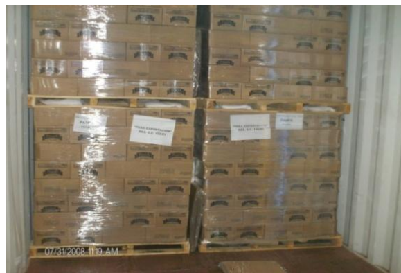
Figure 2-2 Boxes Unitized on Pallets in a Container
