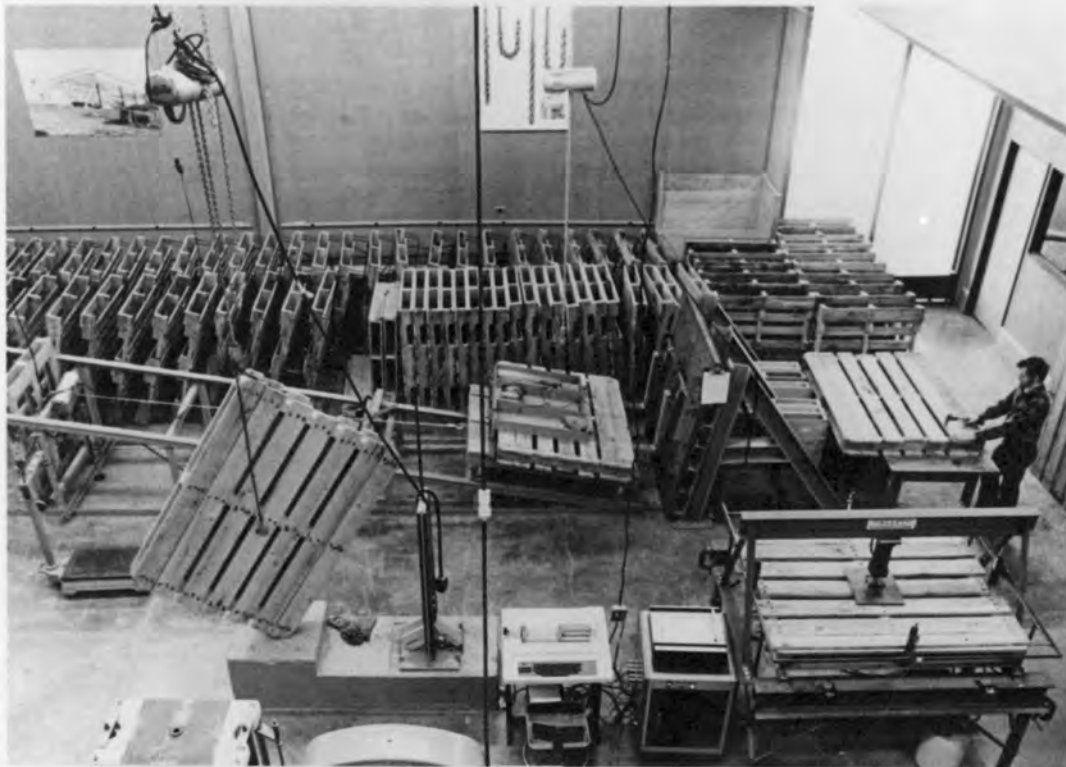
Fig. 4a.- Sequential tests on reversible, double-face, wing-type, two-way, three-stringer, nailed red-oak, 48" x 63", stevedore pallets:
