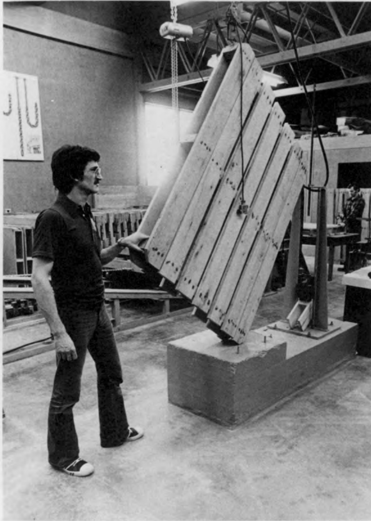
Fig. 4c.- Impact free-fall cornerwise drop test on reversible, double-face, wing-type, two-way, three-stringer, nailed red-oak, stevedore pallet of improved design (held by Nilson Franco).
