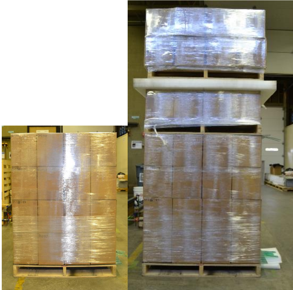
Figure 8 Floor support condition setups for single and double stack unit loads.
