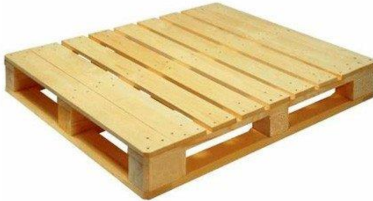
Figure 1 48"x40", Block-Class, Double Face Non-reversible, full four way, stinger board/deckboard top, perimeter base, multiple use pallet.
